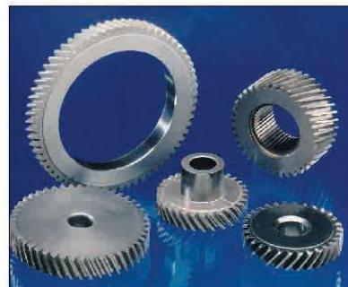
Powder metal transmission gears (made of Cr-Mn-Mo carburizing steel) are carburized using acetylene gas at 900°C (1650°F) to a case depth of 0.35 mm (0.014 in.) and oil quenched. Hardness at the same depth is 500 HV; particle hardness is 700 HV at 40 µm (1600 µ-in.). Photo, courtesy Stackpole Ltd., Advanced Gear Div., Mississauga, Ontario.
