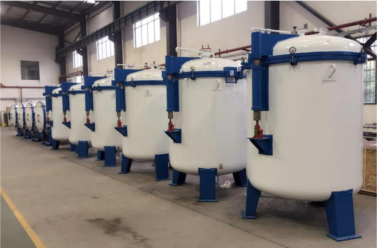
This equipment is mainly applied in sintering and graphitization of carbon materials, carbon fiber rope sintering, high temperature treatment of battery cathode materials, graphite powder, carbon fiber carbonization, high temperature sintering of contact materials, precision ceramics, high temperature component, powder metallurgy materials, tungsten carbide products, etc., and other materials that can be sintering and smelting in carbon environment.
